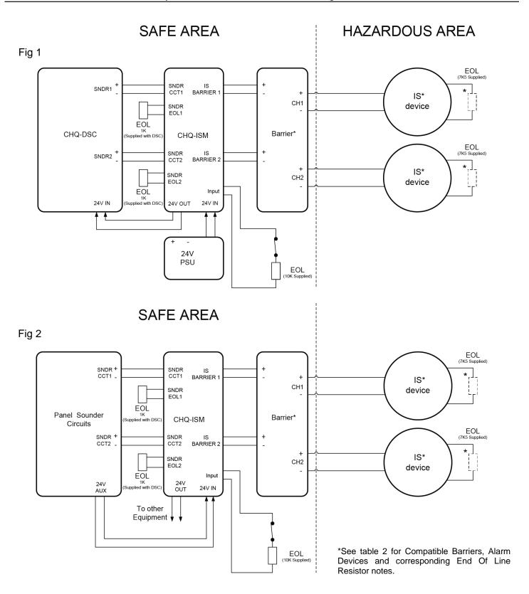
NOTE: For both Fig 1 and 2 a S/C fault on the Barrier terminals will be reported back by the CHQ-DSC or panel sounder circuits as an O/C fault, it will only be reported as a S/C on the CHQ-ISM status LED's.
